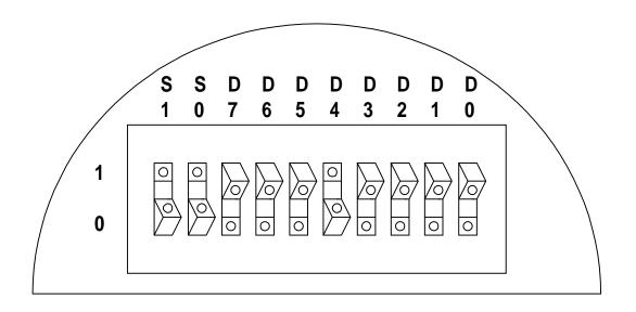
Figure 3. Dip Switches Set to Value 1100010000 to Reset the XRD9829
